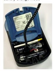
Use the integrated Lithium-Ion battery and continue with 2 standard AAA batteries when the accumulator runs low.
