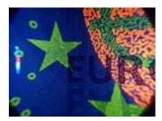
The option UVC equips your Doculus Lumus® with 4x UVC LEDs to view security printings at 254 nm. Compared to the commonly used UVC ring tubes, these LEDs offer the advantage that they provide improved illumination and are not damaged when the device has been dropped (drop-proof 1,5 m).
