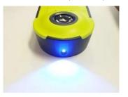
The integrated front UV torch allows to view an entire passport page at a glance with UV 365 nm.
