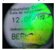
Automatic or manual rotating incident light to the left or right. The rotating incident light (similar to coaxial light) enables the examination of identigrams and holograms through the main lens of Doculus Lumus under magnification.
